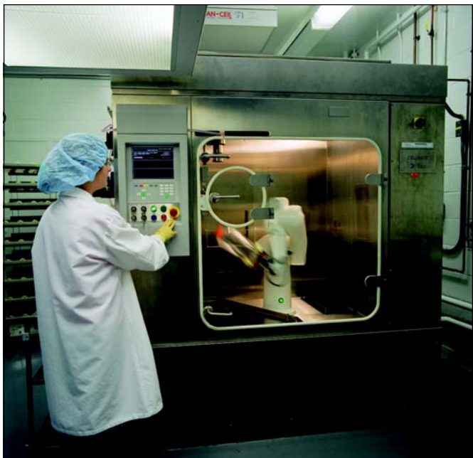
Figure 3. Typical automated roller bottle system for scaled-up production. The robotic arm is capable of handling approximately 1500 roller bottles per batch, based on a single shift per day.
