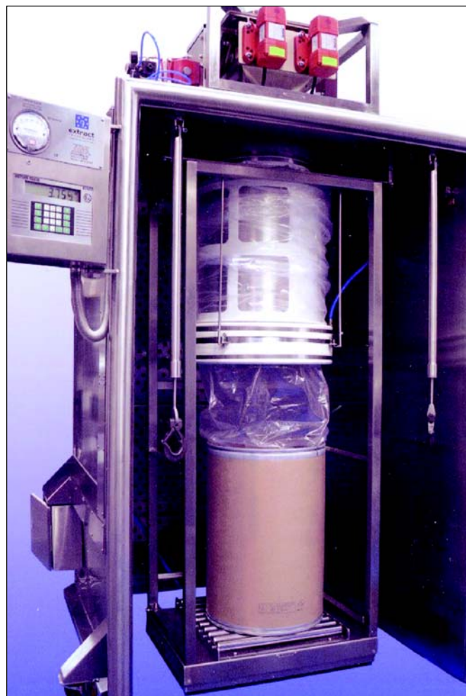
Figure 3. Drum packout head with a continuous liner.
