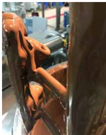
Figure 2: Product residue before initial cleaning step.
