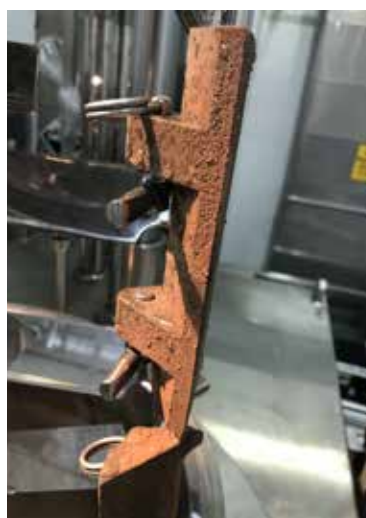
Figure 3: Product residue after initial cleaning step.
