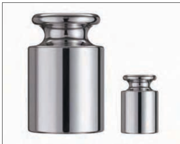
Figure 5. Two test weights are recommended. The large weight has a mass close to the nominal capacity of the weighing instrument, while the small weight amounts to a few percent of the nominal capacity. The large weight is used to test sensitivity and eccentricity, the small for repeatability (if required, together with an additional tare mass).
