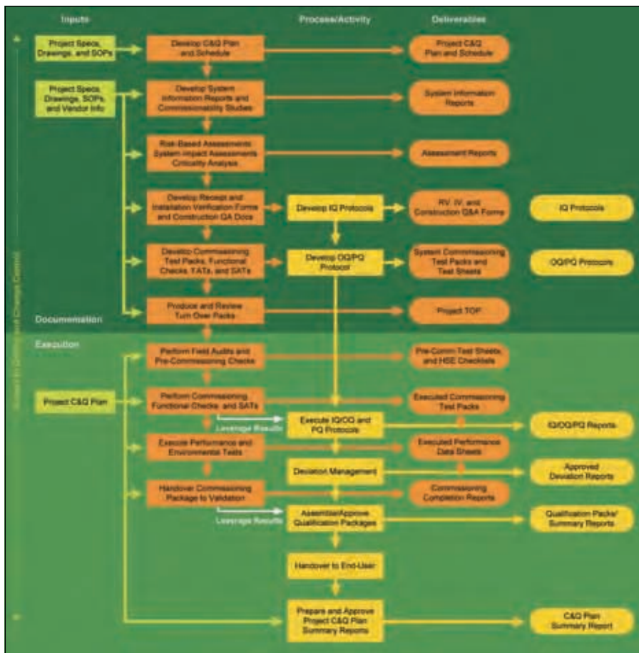
Figure 2. Integrated Commissioning and Qualification (ICQ) flowchart.
