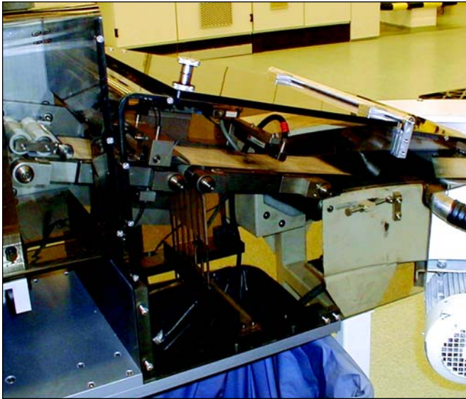
Figure 3. Device used to reject a faulty product – identified during the manufacturing process.
