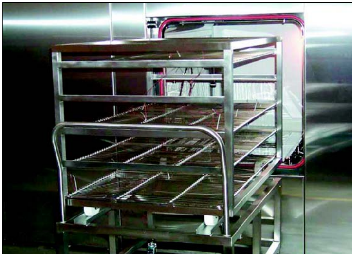
Figure 1. Empty chamber temperature mapping (Photograph provided courtesy of Kuhlman Technologies Inc.)
