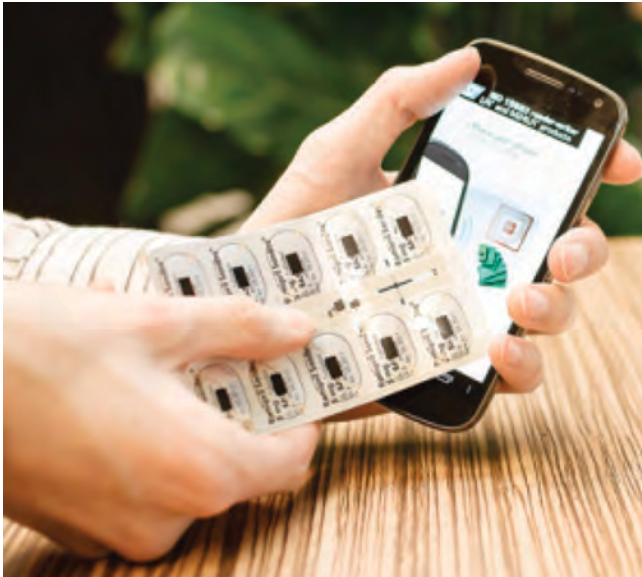
Figure 4. Medication kit with E-Label being read by a mobile device.
